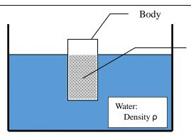
The buoyant force is same as the weight of the water displaced in this area.
