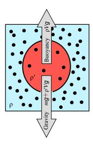
When buoyancy and gravity are in the equilibrium state, the equation is shown as [Upward force] = [Downward force]  $\rho Vg = mg + \rho' \quad Vg$  become smaller when the air heated  $\rho Vg > mg + \rho' \quad Vg \Longrightarrow \text{ float }$   $\rho V > m + \rho' \quad V$   $\rho - \rho' > \frac{m}{V} \qquad \cdots \qquad \boxed{ }$
