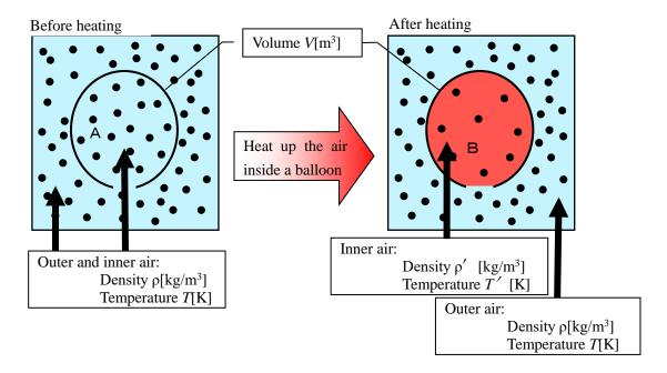
The density of air inside a balloon decreased compared with that of outside, so the net buoyant force works on it.
